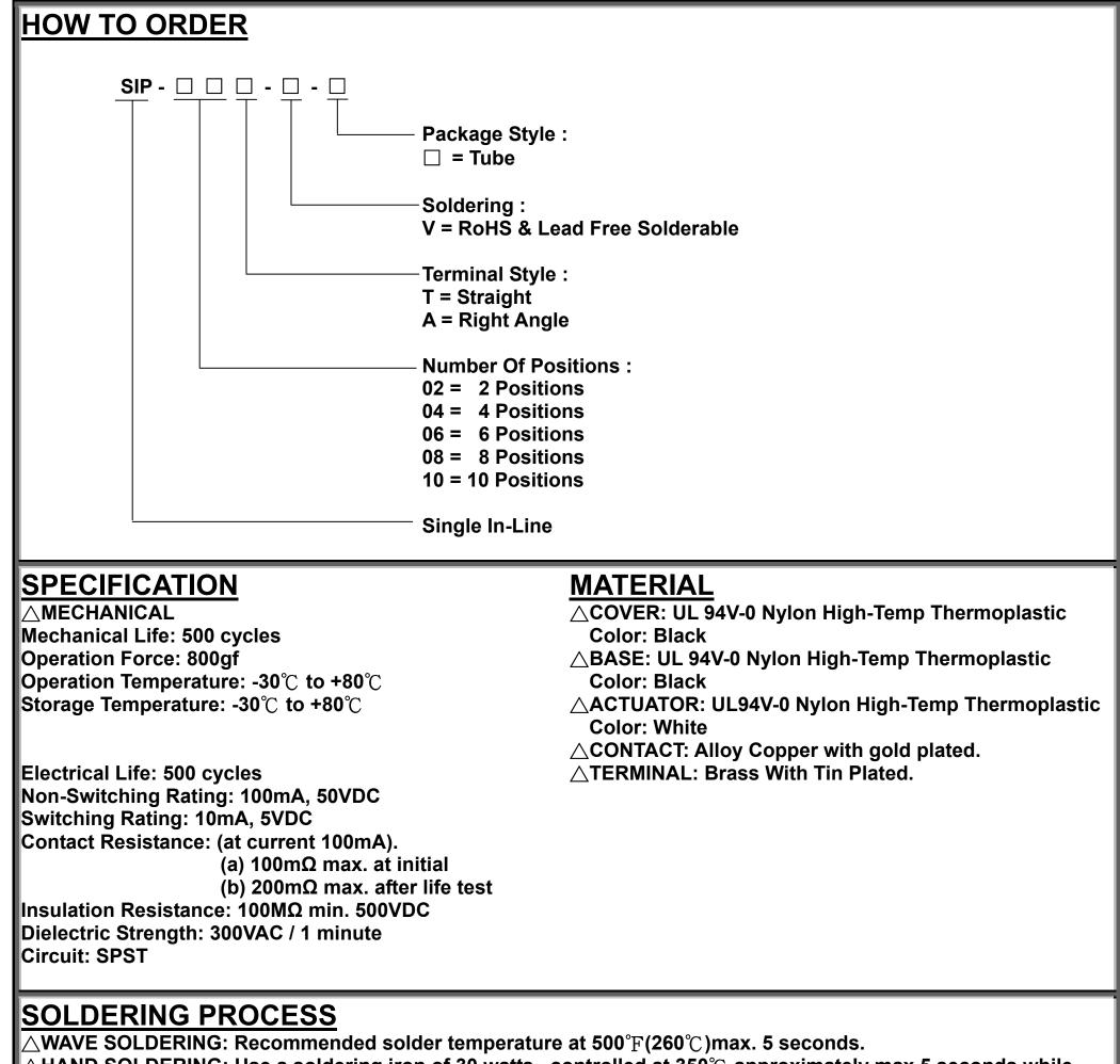
$\triangle$ HAND SOLDERING: Use a soldering iron of 30 watts , controlled at 350 °C approximately max 5 seconds while applying solder.
